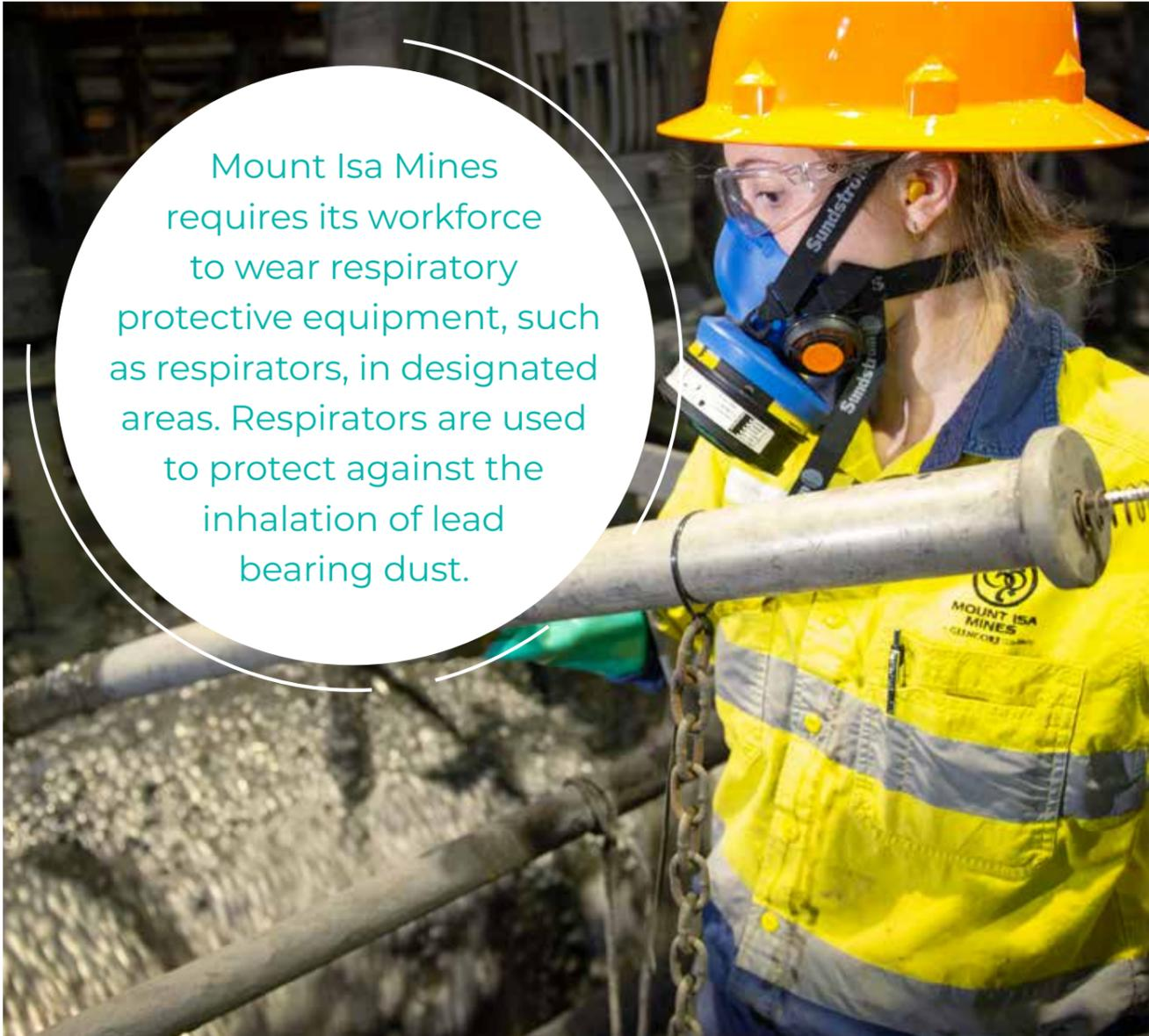
Mount Isa Mines requires its workforce to wear respiratory protective equipment, such as respirators, in designated areas. Respirators are used to protect against the inhalation of lead bearing dust.
