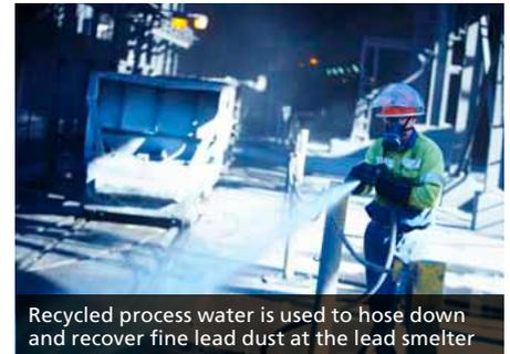
Recycled process water is used to hose down and recover fine lead dust at the lead smelter
